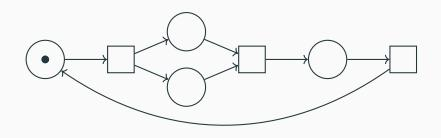
$m \stackrel{*}{\to} m'$  iff  $\exists w : m \stackrel{w}{\to}_{\mathbb{R}_{\geq 0}} m'$  and w(t) = 0 for all t in an unmarked cycle
